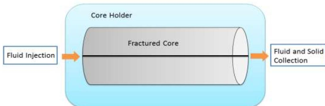
Figure 4. Flow Path inside Core Sample.
