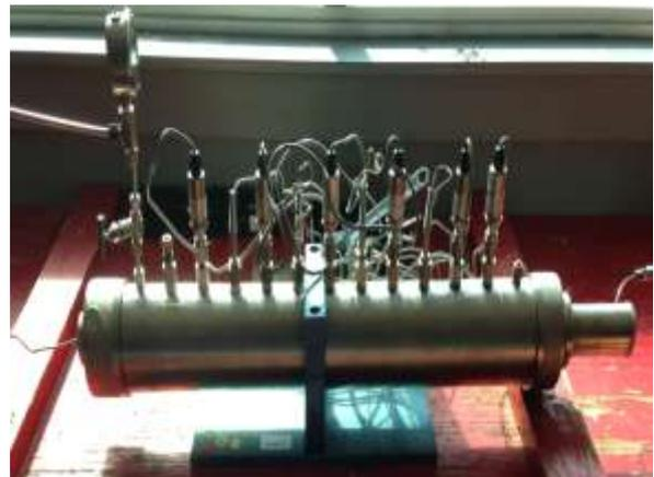
Figure 2. A Hassler Type Core Holder used in the Experimental Investigation.
