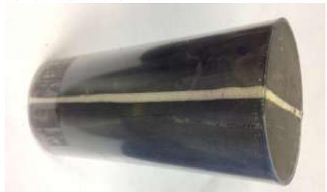
Figure 3. "Fractured" Core Sample with Proppant Inserted.
